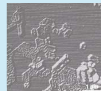
Magnesium chloride crystals on flat silica
