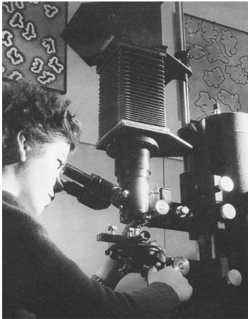
A researcher at AKU's synthetic fibres pilot plant examines the cross-sections of fibres under a phase-contrast microscope.
