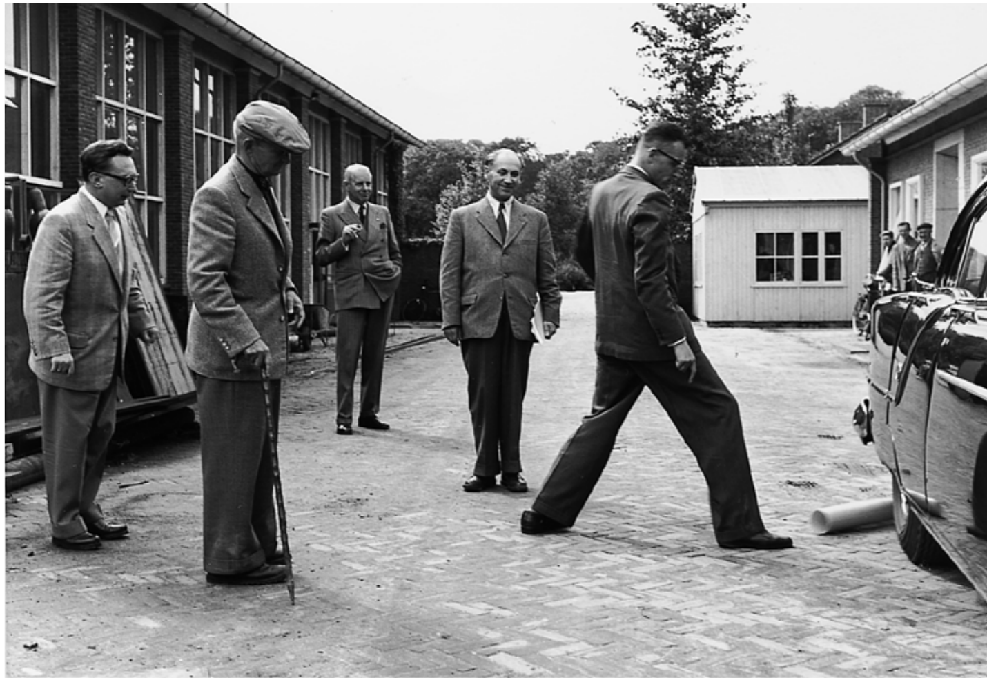
The director of Dutch manufacturer WAVIN demonstrates the shape retention properties of his company's plastic pipes by having a car driven over a water pipe.
